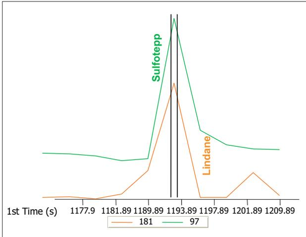
Figure 2. The GCxGC-TOFMS reconstructed 1st dimension chromatogram shows coelution of Lindane and Sulfotepp in the 1st dimension.
