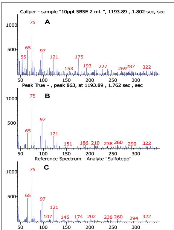
**Figure 5.** Shown in succession is the Caliper-Total Ion Mass Spectrum (A), The Peak True-Deconvoluted Mass Spectrum (B), and the Reference Mass Spectrum (C) for 10 ppt of Sulfotepp spiked in brewed green tea.
