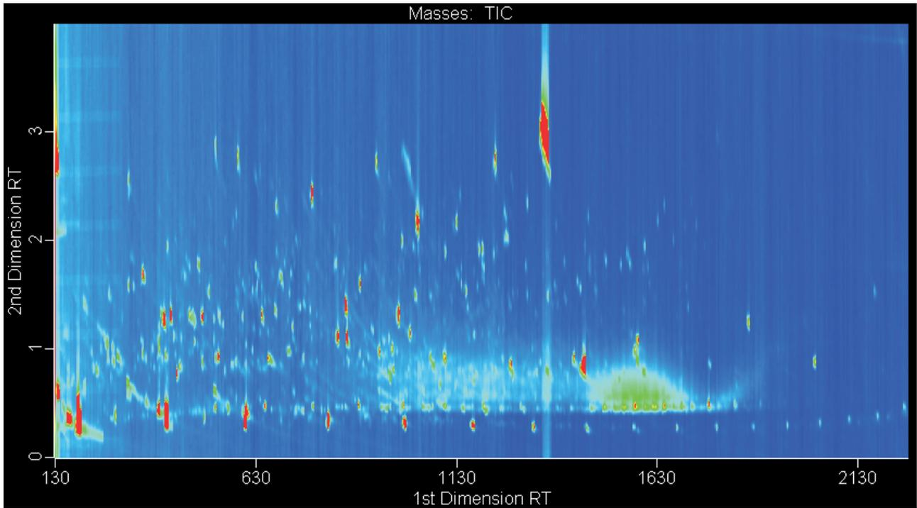
Figure 1. GCxGC-TOFMS contour plot of brewed green tea with OCP/OPP pesticides showing over 1200 peaks at a S/N ratio of 100.
