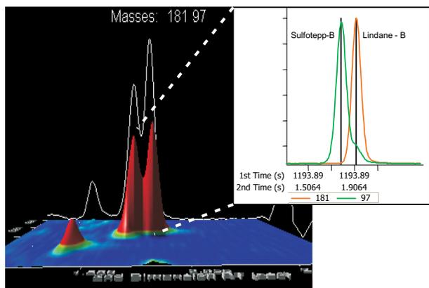
**Figure 4.** The GCxGC-TOFMS surface plot of 500 ppt spiked standards of Sulfotepp (mass=97) and Lindane (mass=181) illustrates the resolution in the second dimension of the chromatographic plane. The inset is the zoomed in linear chromatogram of the modulated slice for the base peaks of Sulfotepp and Lindane. These two pesticides coelute at 1193 seconds in the 1st dimension. However Sulfotepp and Lindane are separated by 132 milliseconds in the second dimension.
