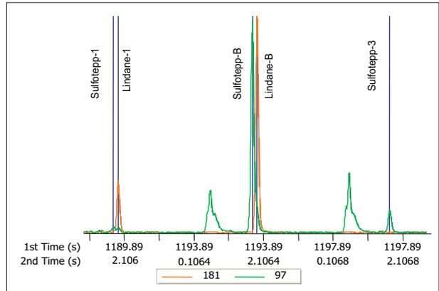
Figure 3. Figure 3 shows that the integration of each slice equals the total area observed in the 3D view. The linear chromatogram shows the uncombined peaks and labelled peak markers for Sulfotepp and Lindane over the GCxGC modulations of 4 seconds each from 1189 to 1197 seconds in the first dimension.
