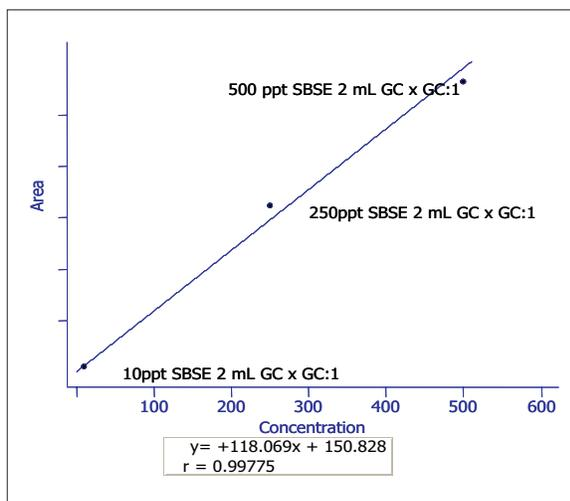
**Figure 6.** Calibration curve for Sulfotepp covering 10 ppt to 500 ppt.
