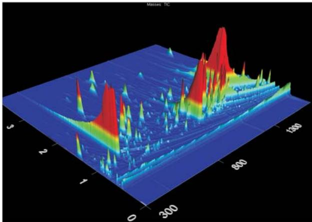
Figure 2. Surface plot of tobacco extract. Retention times for the Rtx-1 separation are plotted along the axis towards the right and retention times for the Rtx-200 separation are shown on the axis going left. A Z-axis represents peak height.
