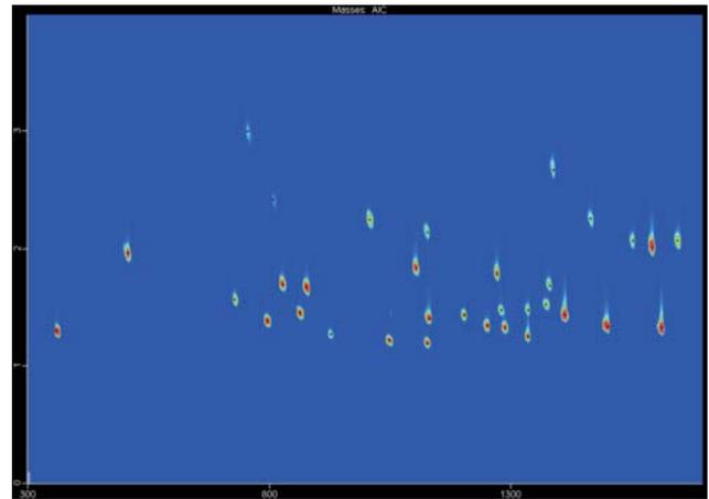
Figure 3. Contour plot of pesticide standard mix analyzed with GCxGC-TOFMS. Note how the pesticides are chromatographed in two dimensions when using the Rtx-1 x Rtx-200 column combination.
