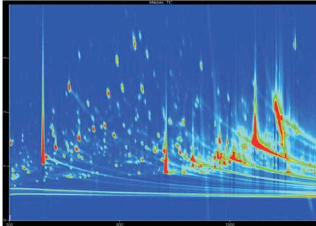
Figure 1. Contour plot of tobacco extract. Retention times for the Rtx-1 separation are plotted along the X-axis and retention times for the Rtx-200 separation are shown on the Y-axis.
