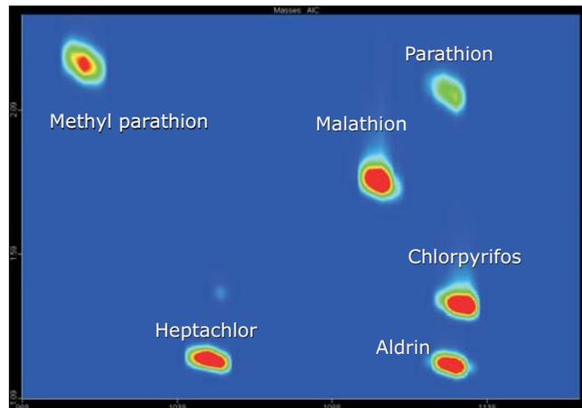
Figure 4. Zoomed in region of contour plot for pesticides standard mix analyzed using GCxGC-TOFMS. The Rtx-200 (the Y-axis separation) provides selectivity to separate Aldrin, Chlorpyrifos, Malathion, and Parathion in the second dimension.
