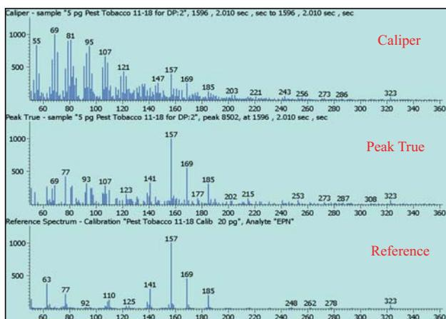
**Figure 10.** Coeluted (Caliper) and deconvolved (Peak True) spectra for the pesticide EPN in a tobacco extract, compared to a Reference Spectrum. The Caliper spectrum represents mainly the coeluting compound or compounds, but the Peak True has an excellent match of 914 against the Reference Spectrum. EPN is at only 5 pg/μL in the tobacco extract.
