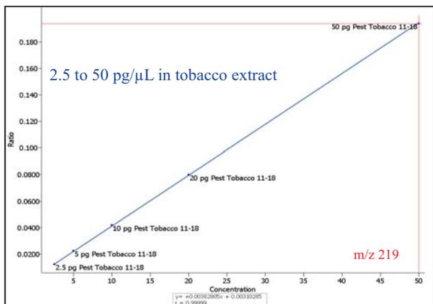
Figure 5. GCxGC-TOFMS calibration curve for gamma-hexachlorocyclohexane (Lindane). The curve was prepared from matrix-matched standards from a tobacco extract.
