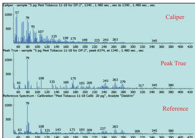
**Figure 9.** Coeluted (Caliper) and deconvolved (Peak True) spectra for the pesticide Dieldrin in a tobacco extract, compared to a Reference Spectrum. The Caliper spectrum represents mainly the coeluting compound or compounds, but the Peak True has a good match of 804 against the Reference Spectrum. Dieldrin is at only 5 pg/μL in the tobacco extract.
