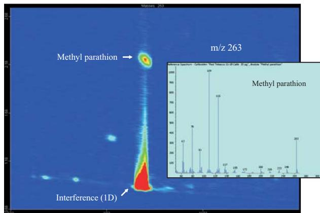
**Figure 7.** The GCxGC contour plot shows methyl parathion resolved in the second dimension on the Rtx-200 column. The quantification mass 263 is plotted. Note the large peak at the bottom of the contour plot that would bias any one-dimensional GC-MS results.
