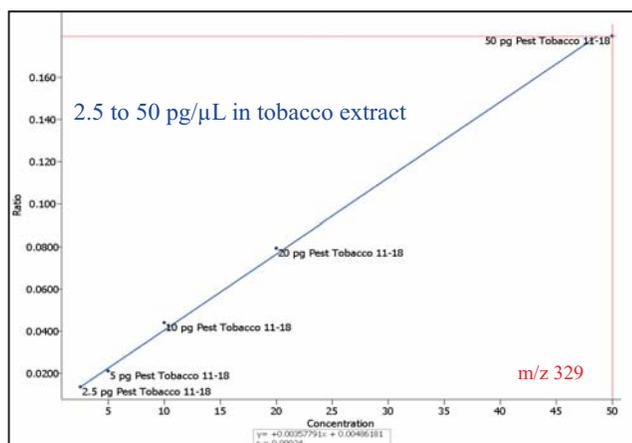
Figure 6. GCxGC-TOFMS calibration curve for Tetrachlorvinphos (Stirophos). The curve was prepared from matrix-matched standards from a tobacco extract.
